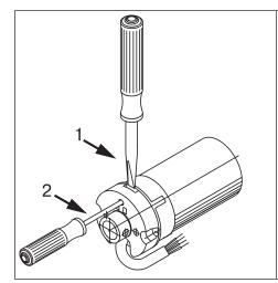
When pushed in, the mounting pin locks automatically. To undo the mounting pin, either insert the screwdriver, max. dia. 2.5 mm, (2) into the hole and push upwards, or push a flat-head screwdriver with a width of approx. 8mm (1) into the groove.
